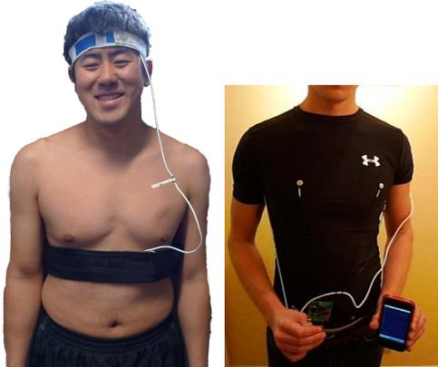
Figure 2: Left: Chest belt containing Tricorder and electrodes, reflective forehead pulse-ox sensor. Right: Compression shirt with conductive fabric on the inside, data visualization on iPhone.
