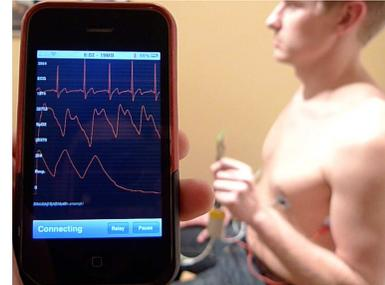
Figure 3: iPhone Bluetooth application. Traces from top: ECG, Red SpO<sub>2</sub>, Respiration Volume
